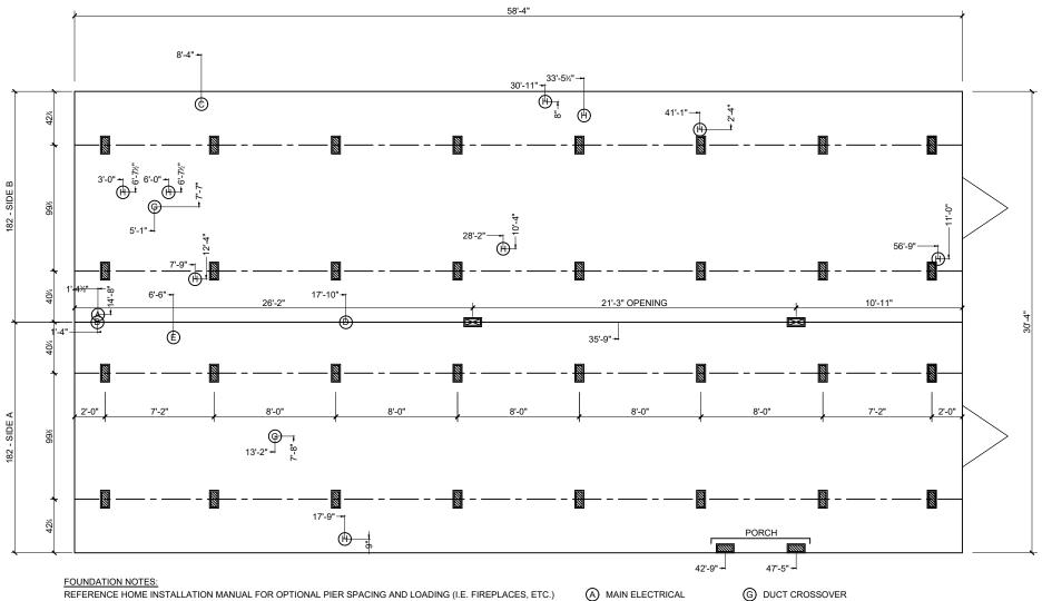
REFERENCE HOME INSTALLATION MANUAL FOR OPTIONAL PIER SPACING AND LOADING (I.E. FIREPLACES, ETC.) SINGLE STACK PIERS MAX. 36" HIGH; DOUBLE STACK PIERS MAX. 80" HIGH. ALL DIMENSIONS ARE FROM REAR OF HOME UNLESS OTHERWISE NOTED.
